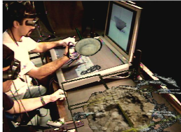
Figure 1. Two users collaborate in VITA. While one user inspects the 3D virtual model of the ceramic vessel above the table, comparing it with the high resolution image on the screen, the second user looks at the 3D miniature terrain model next to the table. (Captured live, using a tracked video-see-through display.)
